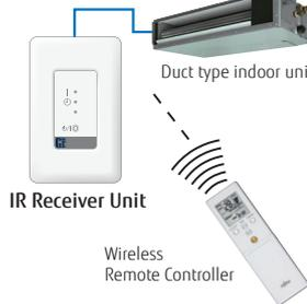
**Duct type\* indoor units can be controlled with Wireless Remote Controller**
